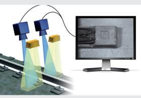
Principle structure of a CrackCheck System
