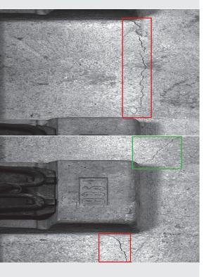
CrackCheck is an automatic inspection system, which checks concrete sleepers and the "slab track" for cracks at high speeds of more than 100 km/h and produces a rail condition protocol as a result, which generates an objective status of the inspected rail for the user with high quality and safety in the shortest time. Using the latest image processing technologies CrackCheck ensures that the rail bed structure inspection is faster, safer and more reliable.
